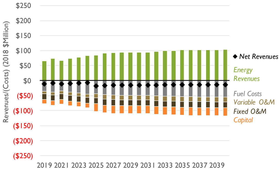
Figure 9. Spruce Unit 1 projected revenues and costs with SCR, AEO low gas price assumptions, 2019-2040
