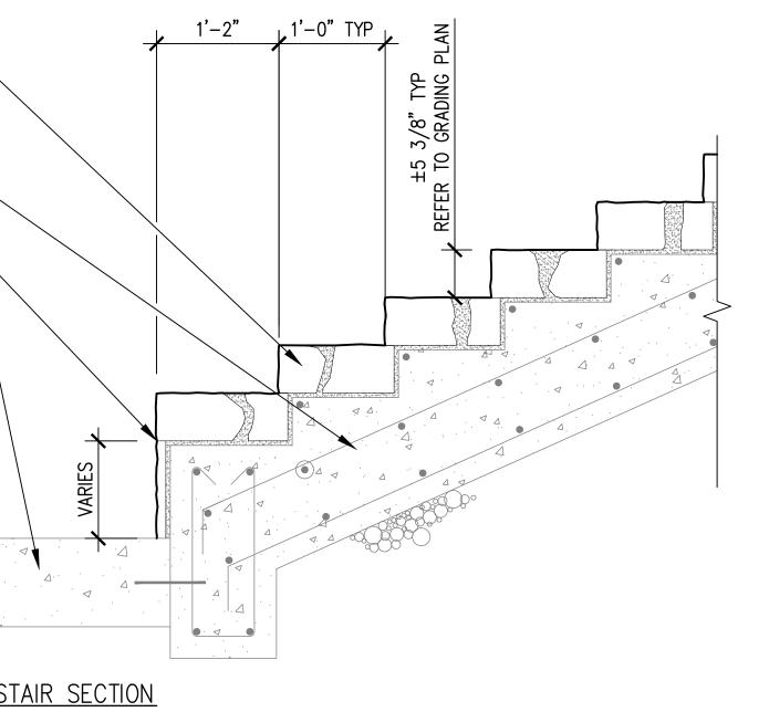
MORTAR SET LIMESTONE COBBLE STEPS -ALL RISERS TO BE EQUAL HEIGHT REFER TO MATERIALS SCHEDULE FOR COLOR AND FINISH
