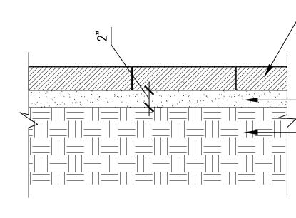
REPLACED PAVER (TYP.); MATCH PAVER SPACING TO EXISTING PAVERS
