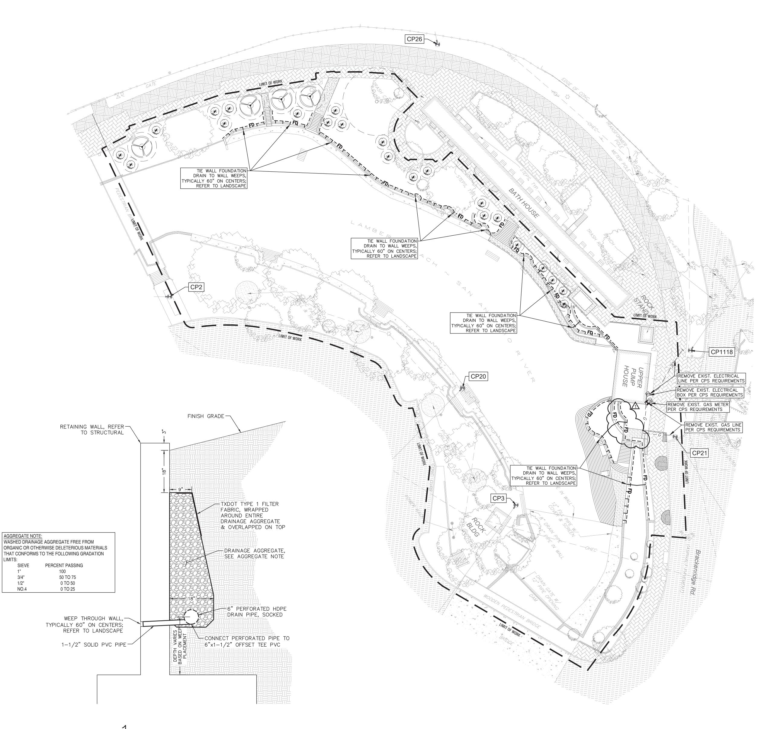
WALL FOUNDATION DRAIN DETAIL NOT TO SCALE
