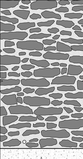
$O3 \xrightarrow{\text{DETAILS} - (WO3) \text{ NEW STONE WALL WITH COBBLE AND CONC. REINFORCEMENT}}{3/4" = 1'-0"}$
