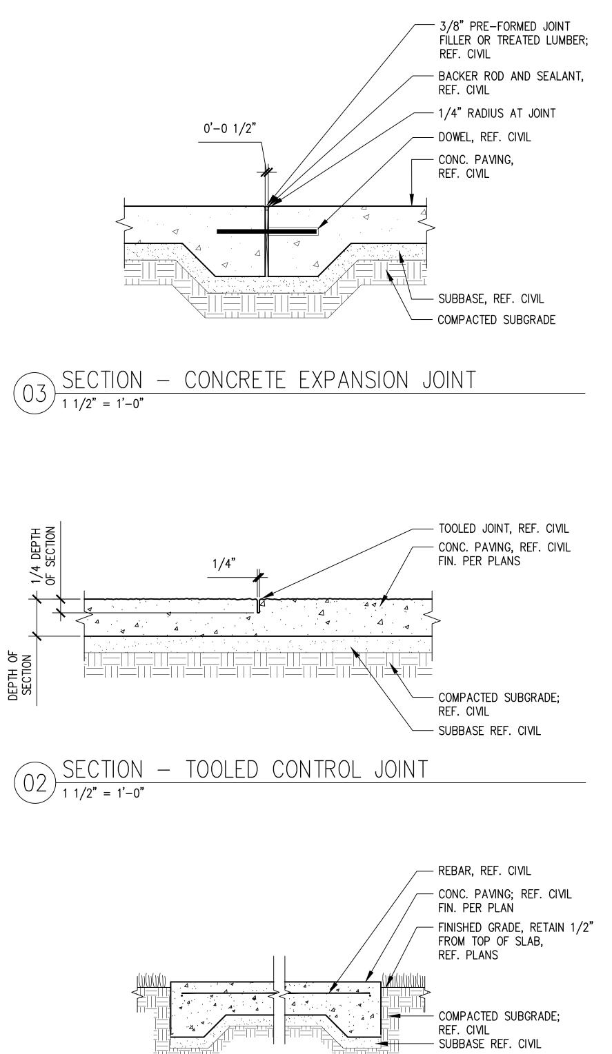
$(01) \frac{\text{SECTION} - \text{TYPICAL CONCRETE PAVING}}{1" = 1'-0"}$
