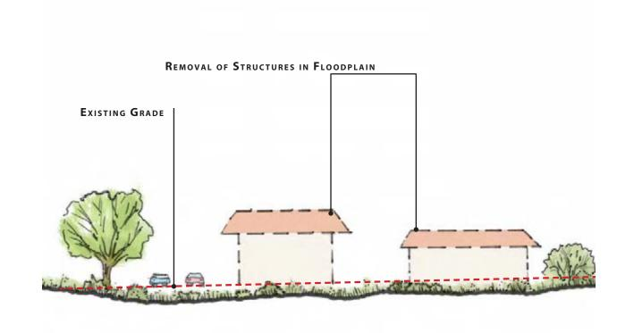
Figure 24. Martínez Creek Proposed Cross Section, Downstream of Cincinnati Avenue
