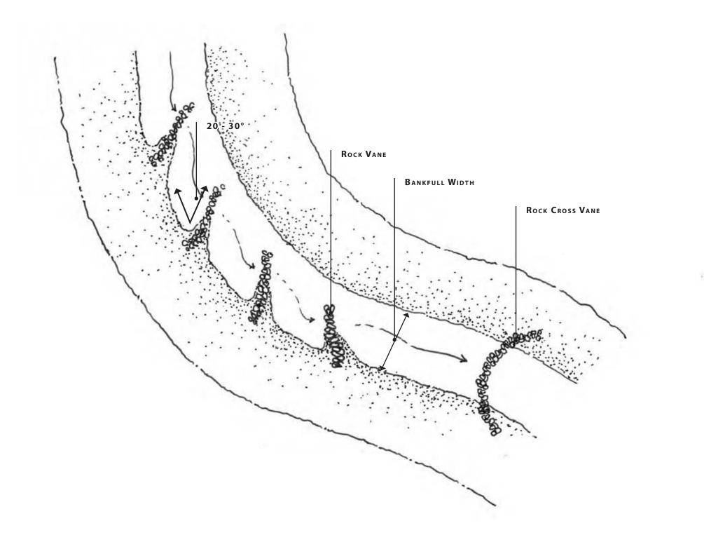
Figure 10. Use of Rock Vanes to Protect Outside Meander Bends
