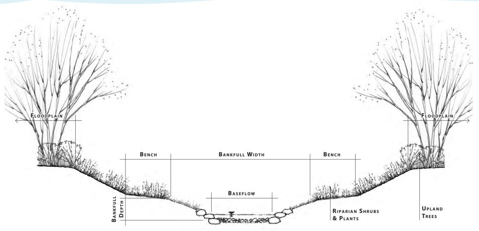
Figure 2. Typical Natural Channel Cross Section
