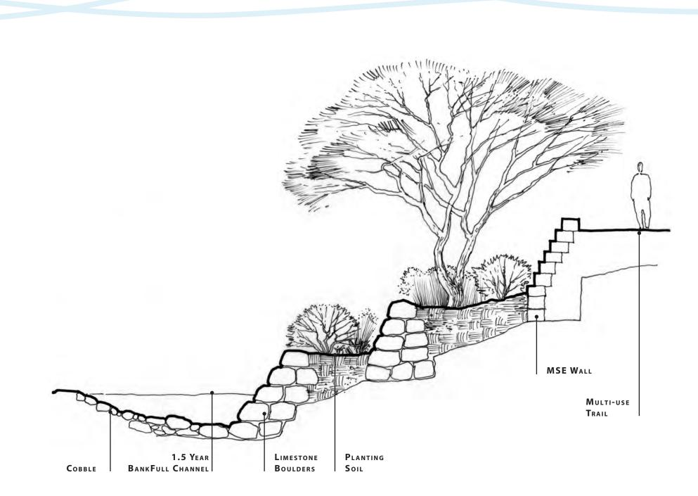
Figure 19. Terracing provides opportunity for soil infiltration and providing greater opportunity for use by down slope plants.
