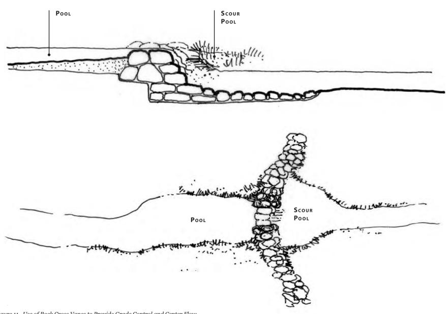
$Figure \ {\tt 11.} \ Use \ of \ Rock \ Cross \ Vanes \ to \ Provide \ Grade \ Control \ and \ Center \ Flow$
