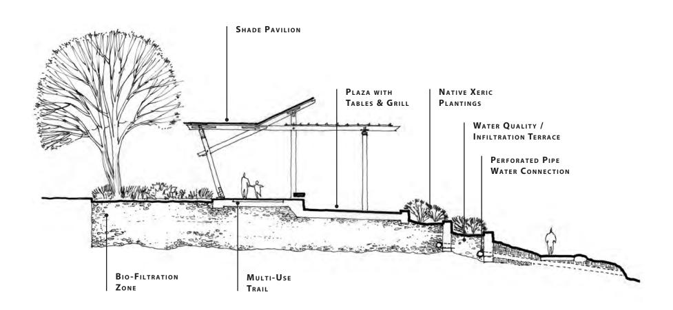
$\label{eq:Figure 20.Bio-Filtration\ allows\ for\ natural\ processes\ to\ clean\ runoff\ before\ entering\ the\ streams.$
